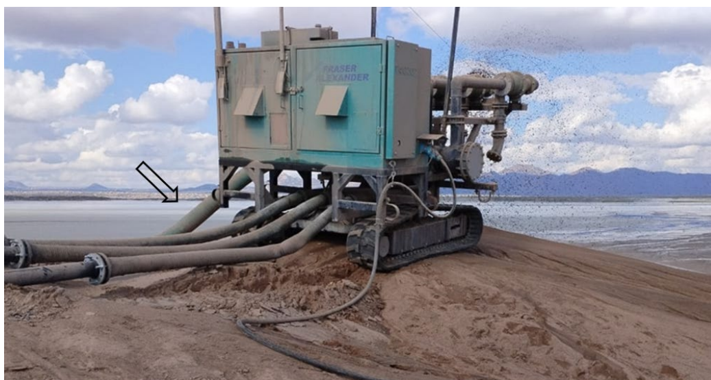
Figure 4: Self Propelled Cyclone Unit Operating at BW1
