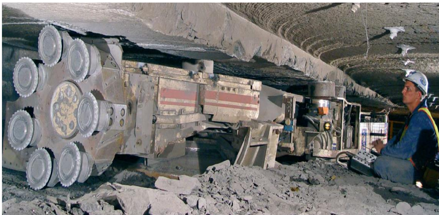
MN220 Reef Miner: Remote controlled disc cutting machine designed for mining narrow reefs of hard rock
