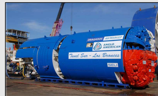
Tunnel Boring Machine
