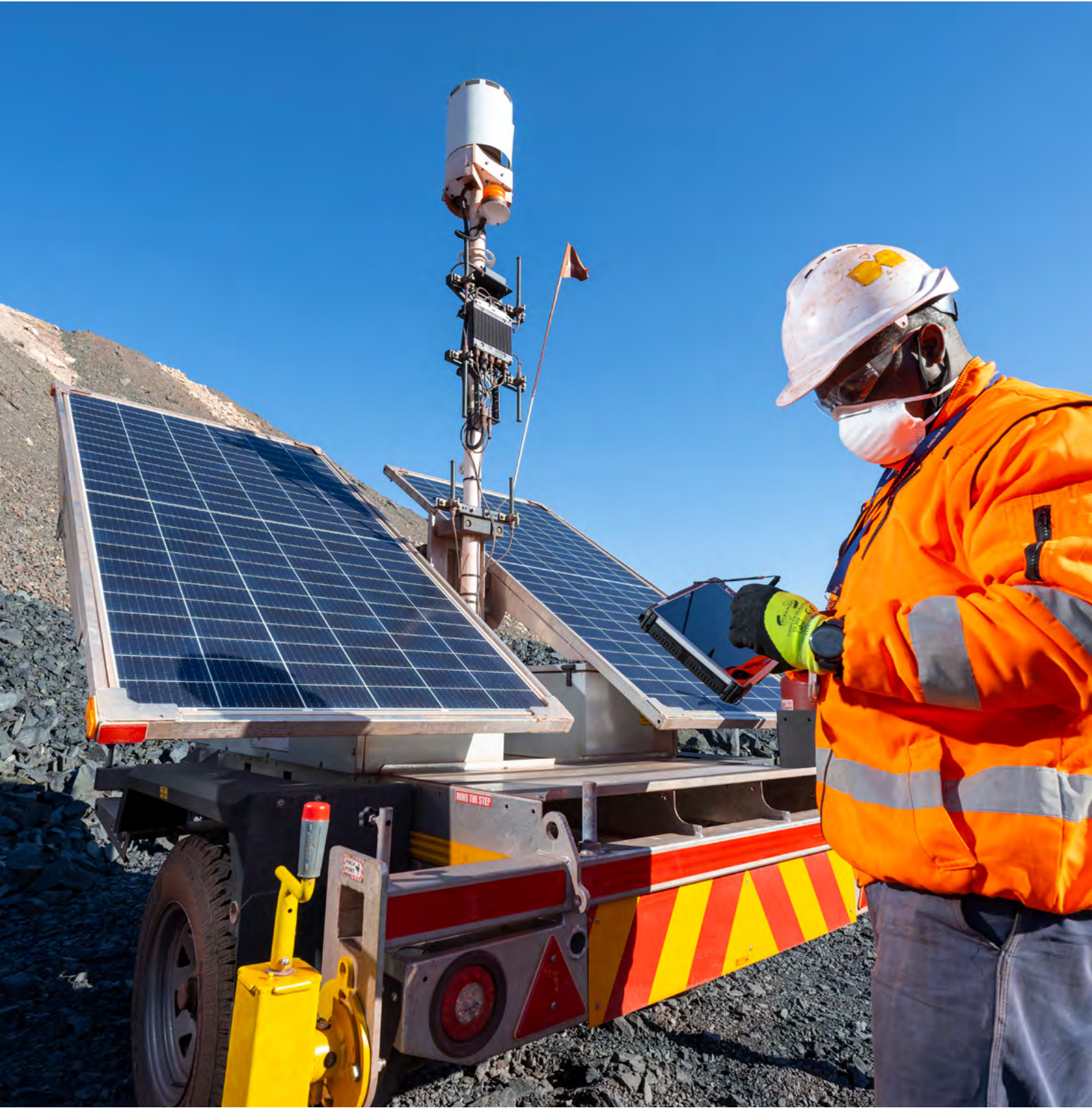
▲ At Kolomela iron ore mine in South Africa, technician Moses Murefu inspects the berm-monitoring system, which monitors any movement or height deficiencies in the berms, and is partially powered by solar power.
