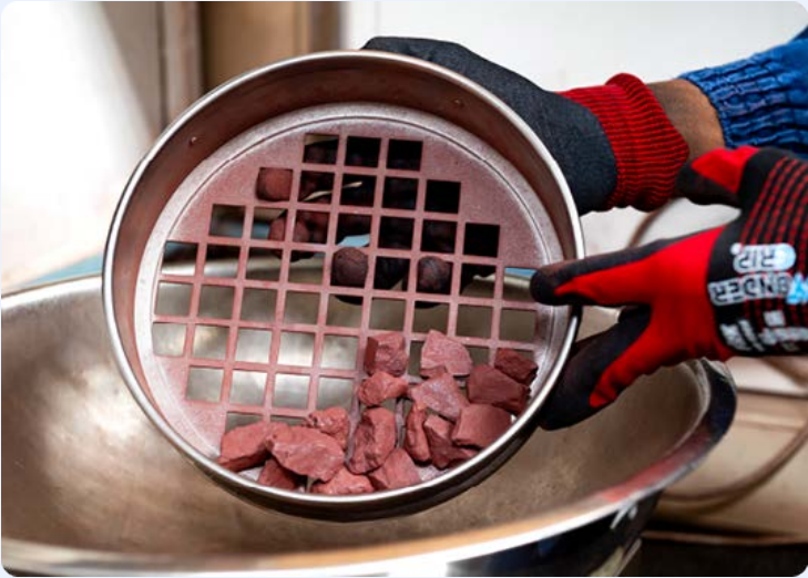
A sample of Kumba Iron Ore's DR Lump product after it has emerged from the screen plant, where the iron ore is reduced in size.
