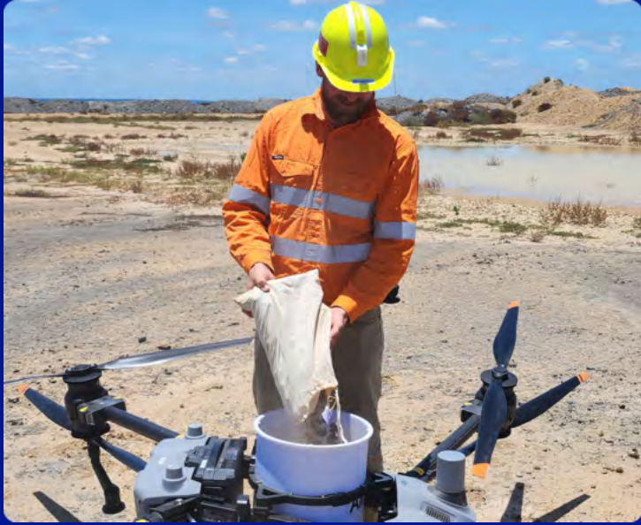
At a Steelmaking Coal site in Queensland, Australia, land stewardship and rehabilitation lead Todd Bell loads a drone with seed pods to be scattered over rehabilitated land areas.
