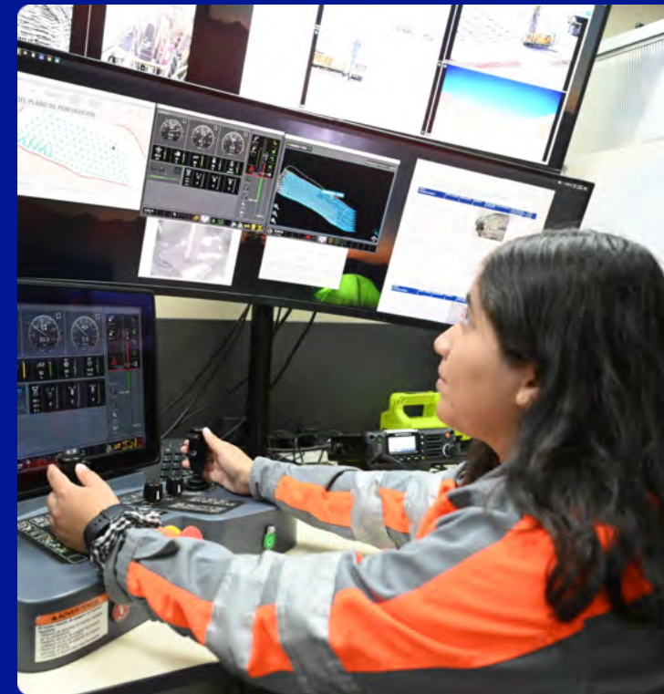
Tania Alvarez Pulleches supervises drilling and blasting operations at Quellaveco from the safety of the Integrated Operations Centre (IOC), six kilometres away from the blasting area.
