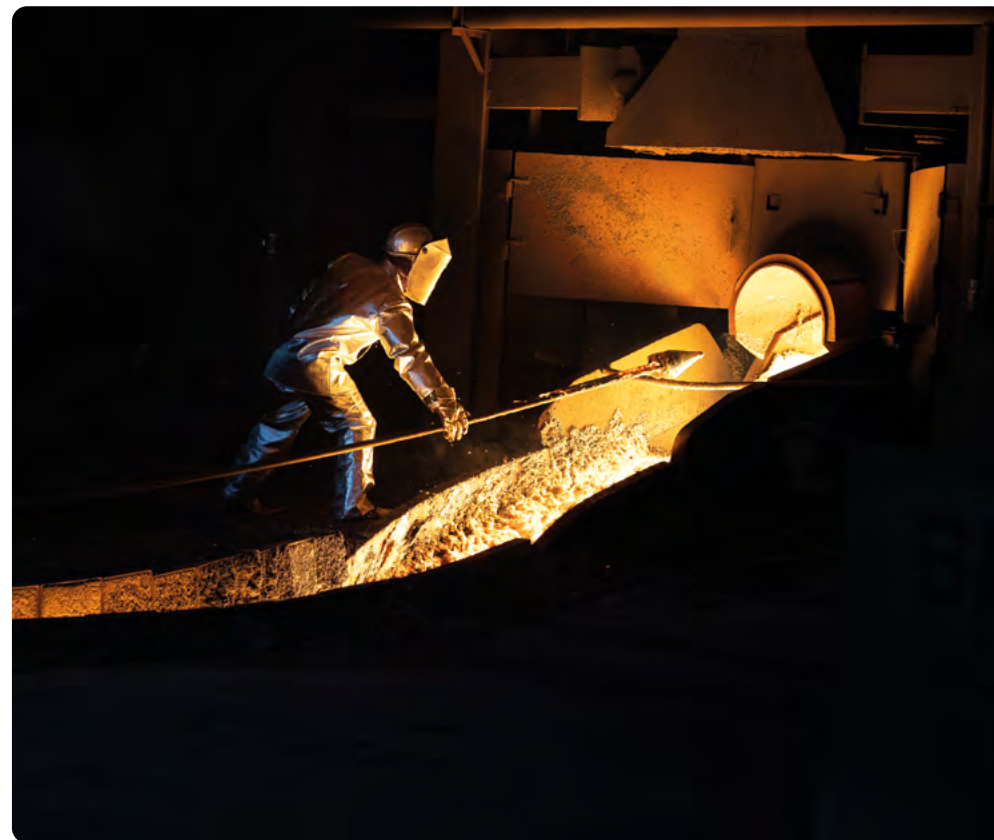
Molten metal is poured from a furnace at our Barro Alto operation, an important producer of ferronickel for the stainless steel industry.
