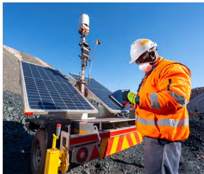
Technician Moses Murefu inspecting the berm monitoring system at Kolomela iron ore mine in South Africa, which monitors any movement or height deficiencies in the berms, and is partially powered by solar power.
