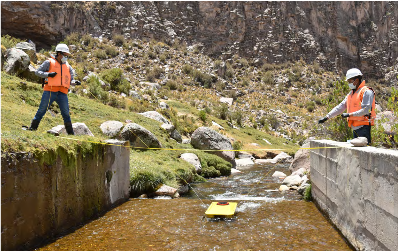
↗ Environmental consultants perform flow measurements at the Asana river, close to our Quellaveco copper project in Peru.
