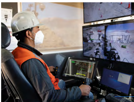
At Los Bronces, major services operator Hector Rojas Soto monitors drilling and blasting operations from the safety of a control centre.
