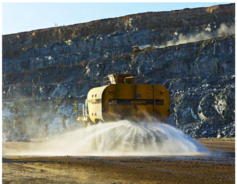
On our mines, dust suppression on roads, waste dumps and crushing operations is a vital daily activity in helping to reduce the amount of airborne particulate material. Here, in PGMs' Mogalakwena North's open pit, dust is controlled through regularly spraying the surface area with a dust suppressant and recycled water.
