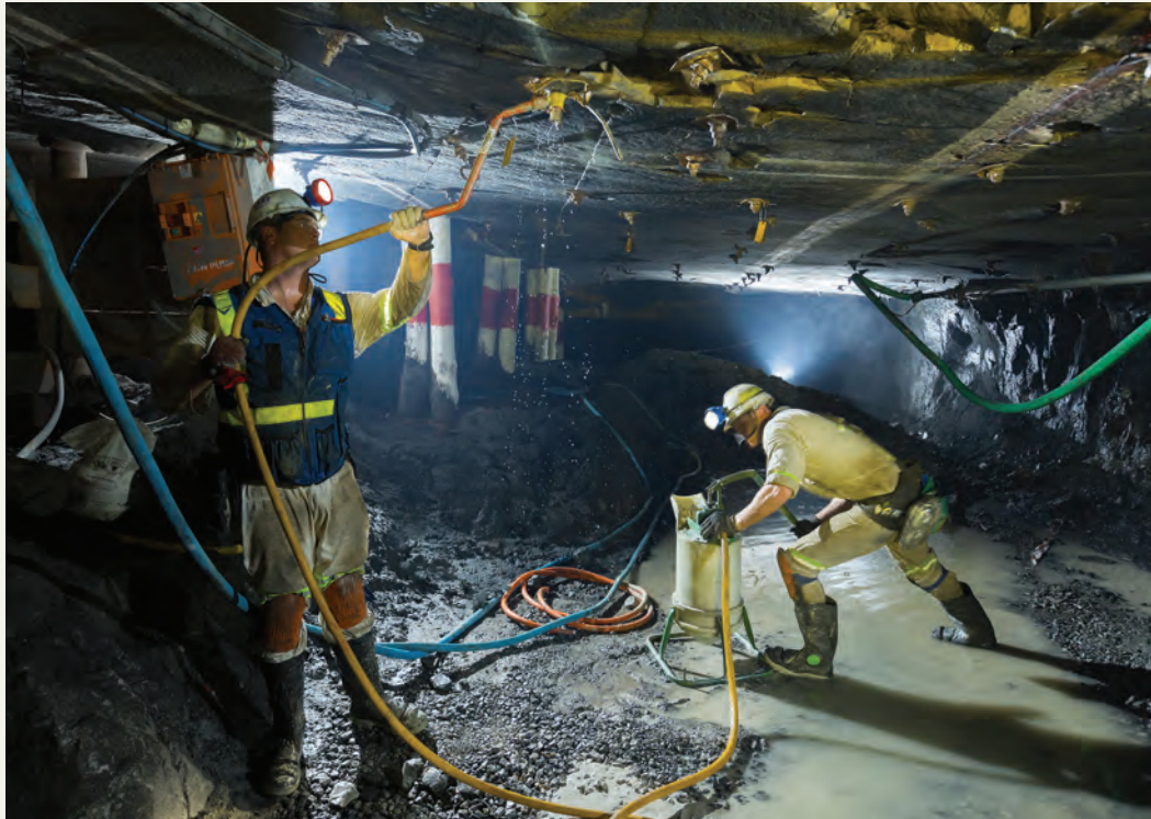
Installation of a flexibolt at Bathopele Mine.
