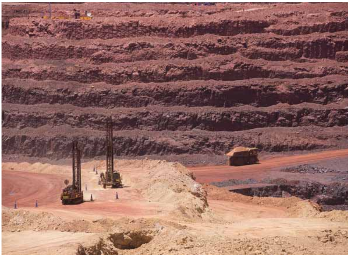
02 A block being prepared for blasting in the Leeuwfontein pit at Kolomela mine.
