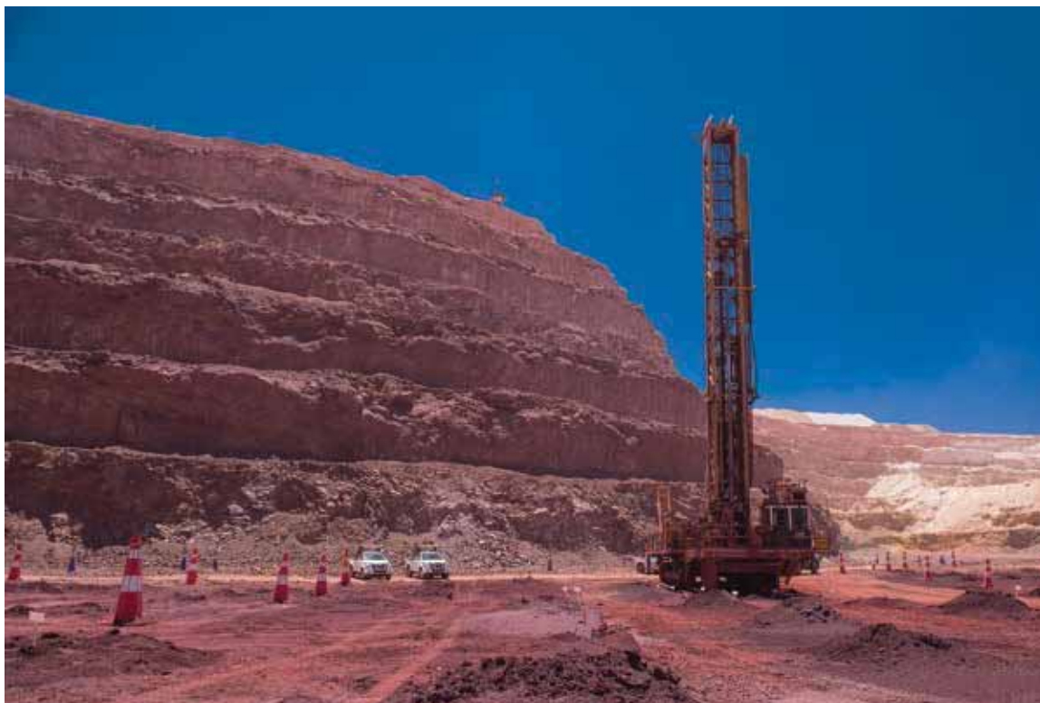
01 Holes drilled for blasting are demarcated by plastic cones in the Leeuwfontein pit at Kolomela mine.
