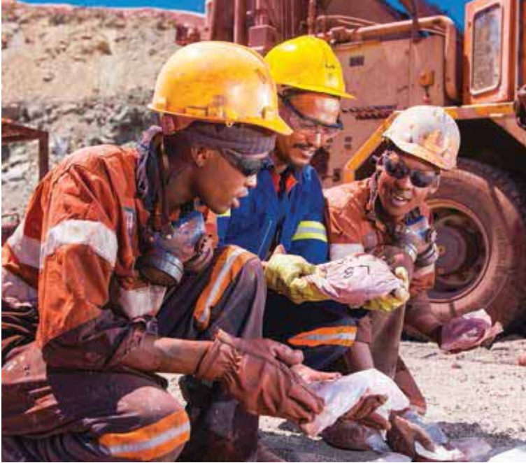
01 Gladwill Gaitswe, Godfrey Montsha and Issac Mongale take ore grade – control samples in the Leeuwfontein pit at Kolomela mine.
