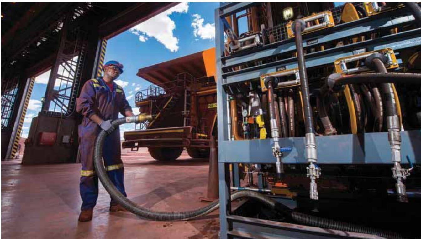
01 Macdonald Mbonani, a millwright at Sishen mine, working in a lube station in the new workshop for mega-class equipment.
