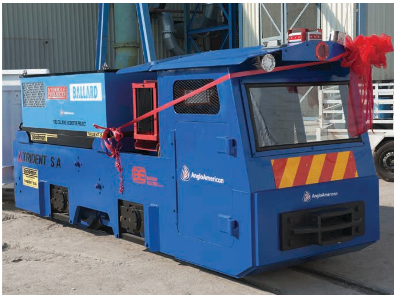
▲ 01 Platinum unveiled a platinum-based fuel cell powered mine Locomotive prototype at Khomanani mine.
