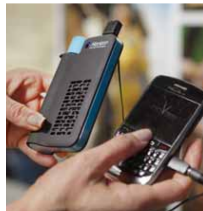
Fuel cell charging a cellular phone
