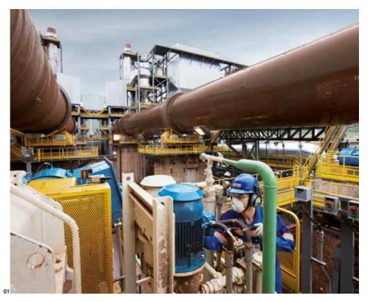
01 At Barro Alto, ore is heated at very high temperatures in these two 185 metre rotary kilns in a process known as calcining, which removes moisture and water crystals from the nickel bearing ore and starts the metallurgical process.
