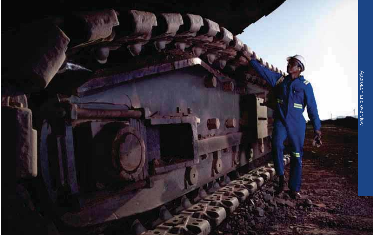
Nelson Sepaela, shovel operator, performing a pre-shift inspection on a shovel at Thabazimbi mine.
