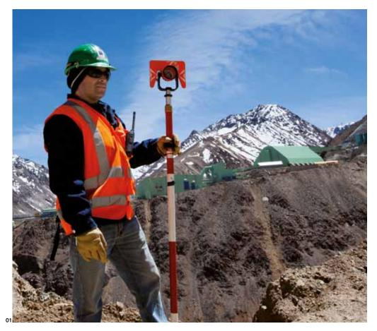
01 Taking topographical measurements at Confluencia, with the new stockpile building in the background.
