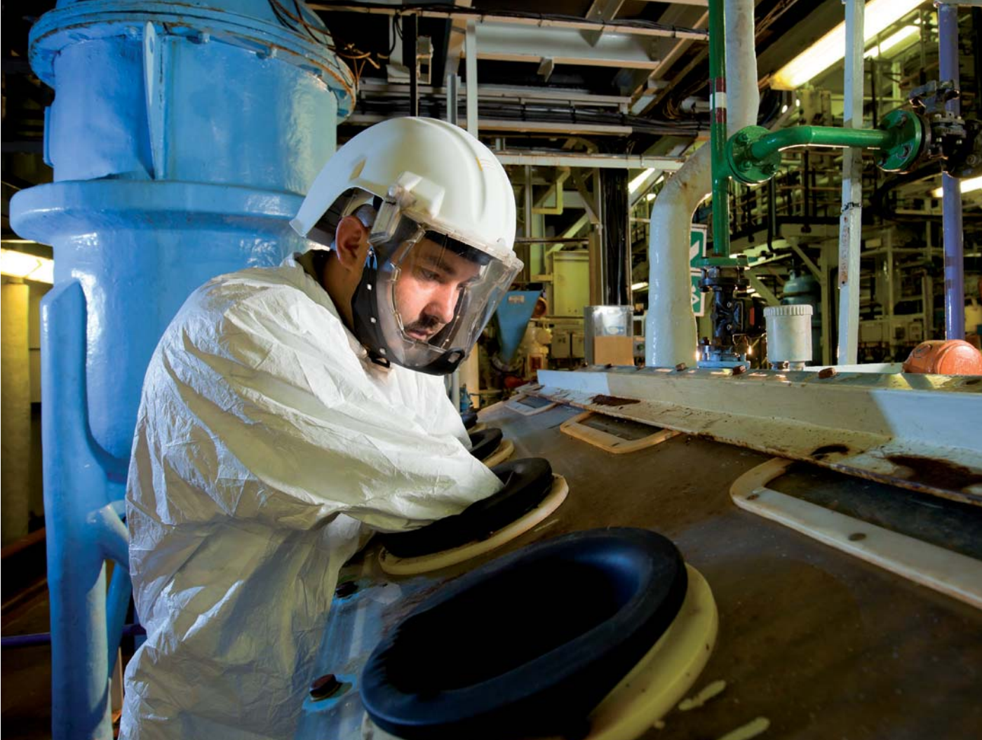
Hannes Jordaan removes platinum residue from a glove box filter at PMR.
