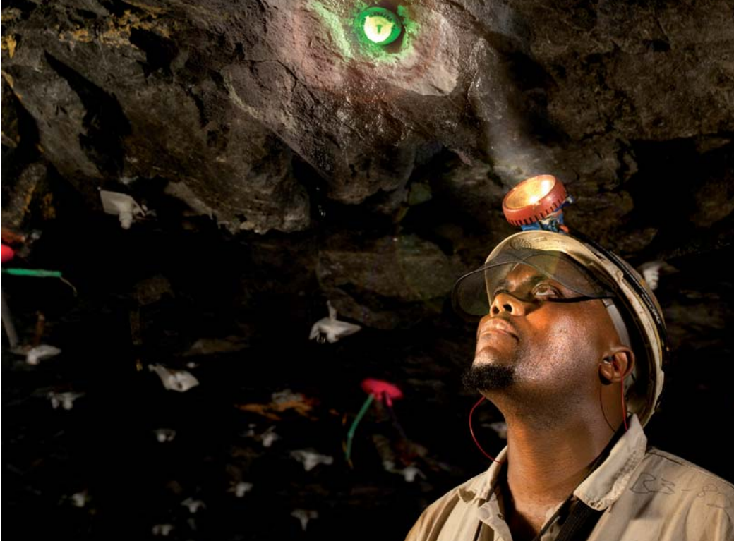
Sydney Mabale observes a fall-of-ground light installed to monitor ground movement.
