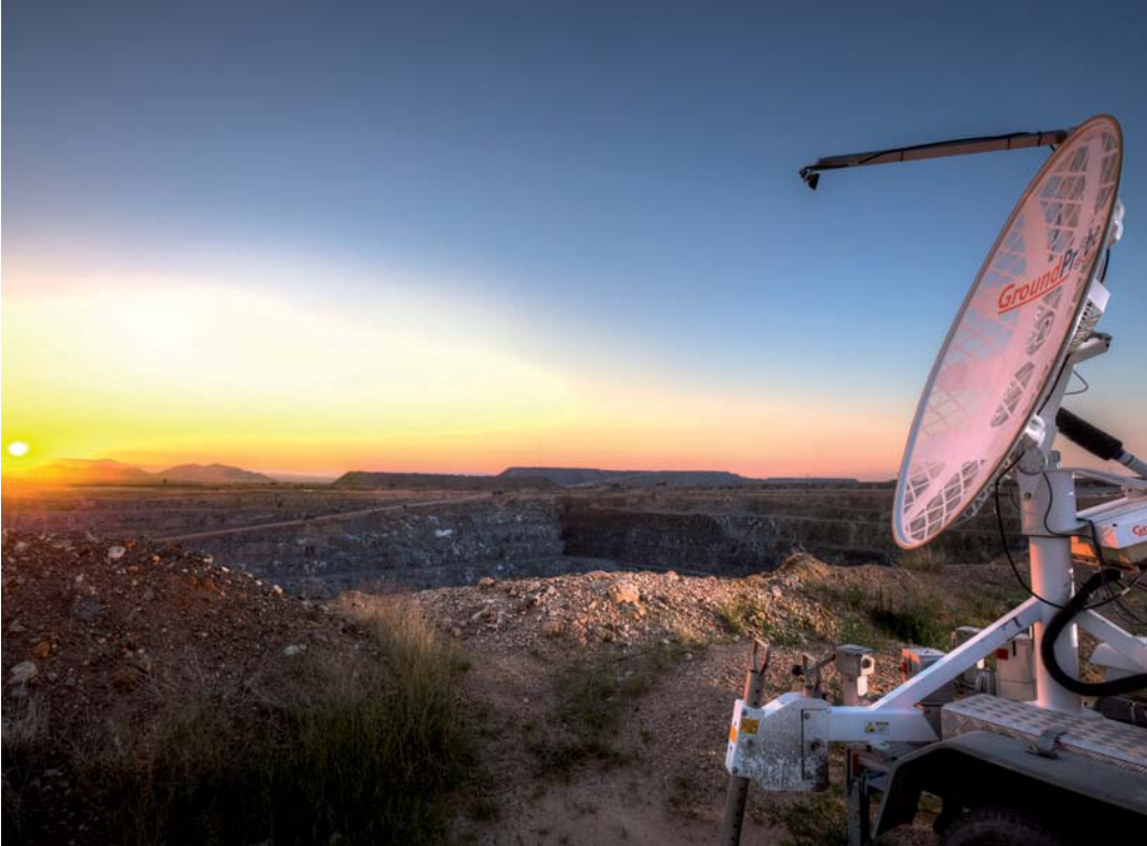
Slope stability radar in use at Mogalakwena Mine.
