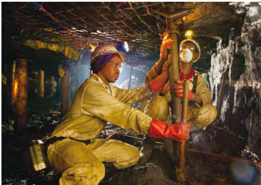
Employees inspect in stope safety netting which has been installed as standard in all underground operations at Anglo Platinum to reduce incidents from falls of ground
