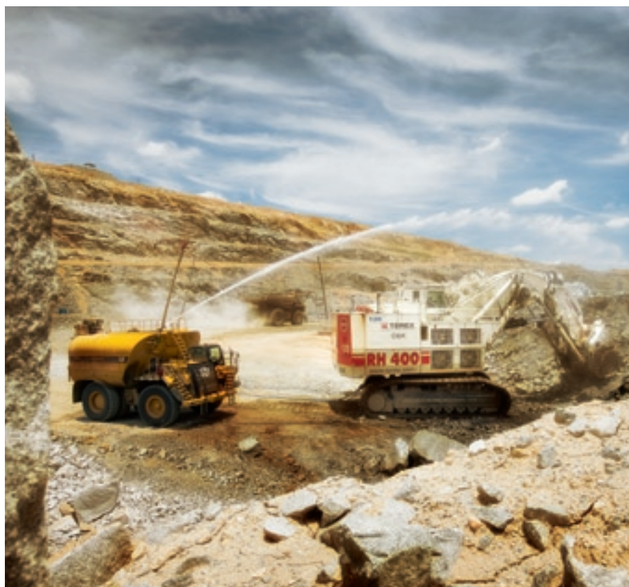
At Anglo Platinum's Mogalakwena open pit in South Africa, a water cannon suppresses dust during ore loading operations.
