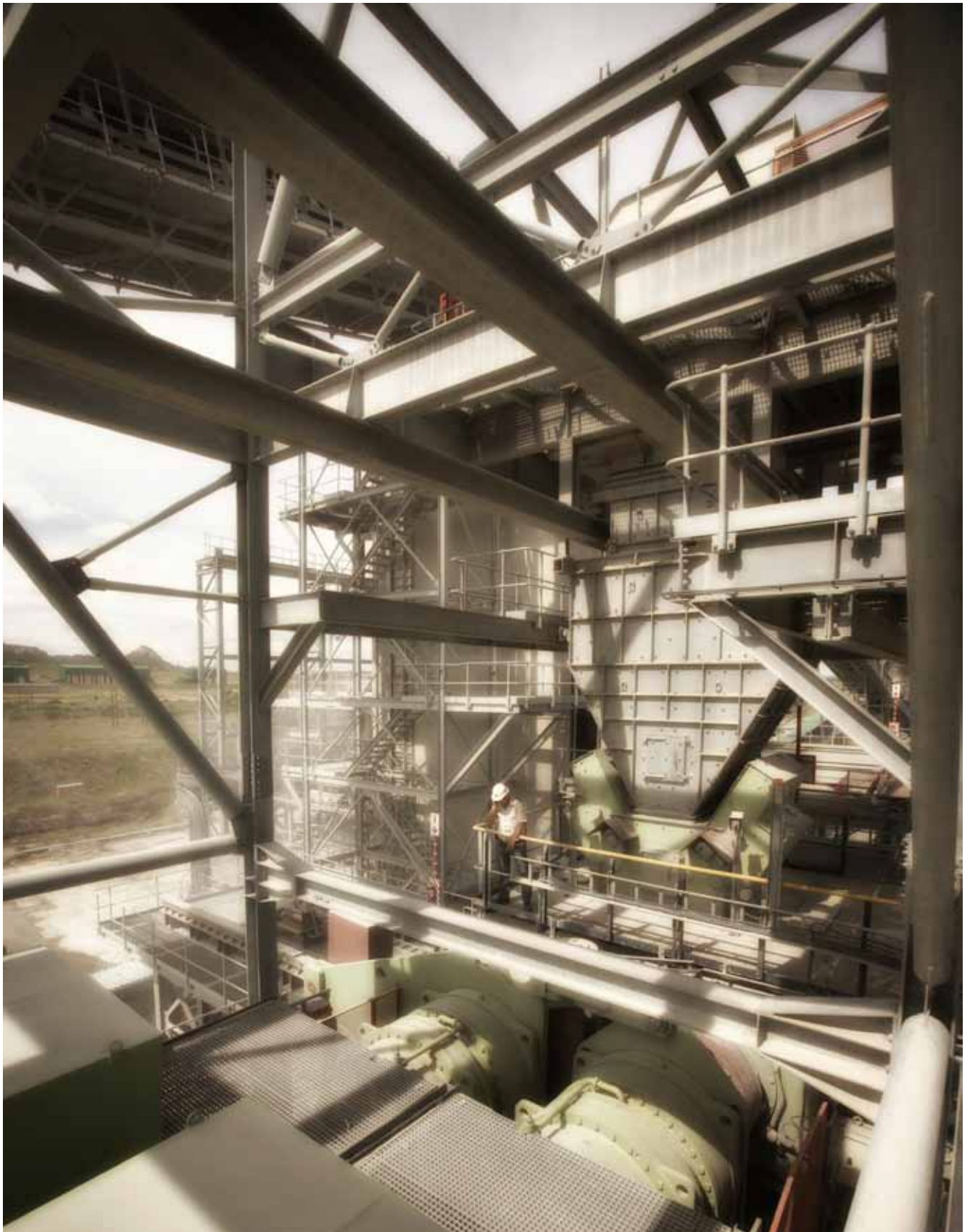
Energy efficient high pressure grinding rolls that are 20% more efficient than traditional mills
