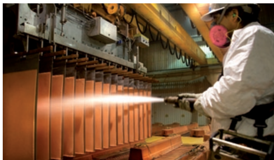
Washing copper cathodes at the San Francisco cathode plant in Los Bronces
