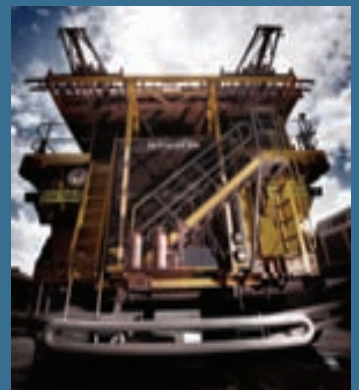
Top: Safety Through the Empowerment of People (STEP). Middle: Kumba acknowledges the importance of bold signage to remind employees of their duties. Bottom: This truck, at Sishen Mine, is fitted with a safety bumper and collision avoidance system.
