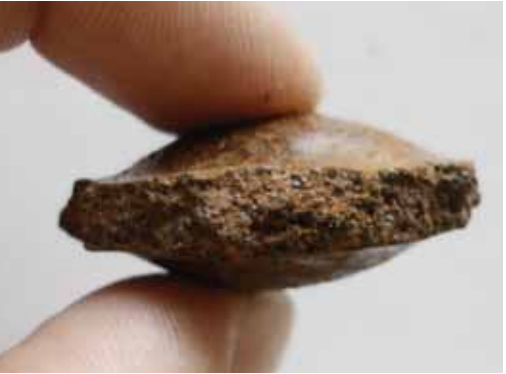
> An environmentally-friendly briquette produced through a reclamation process at CWI.
