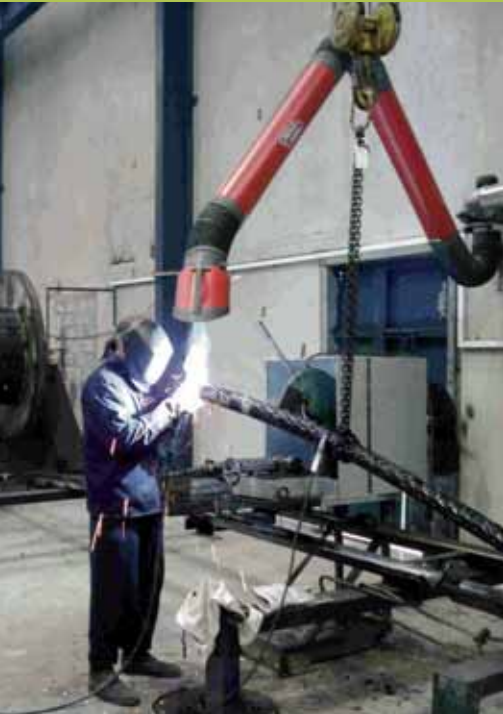
> Fume extraction system in operation during welding.
