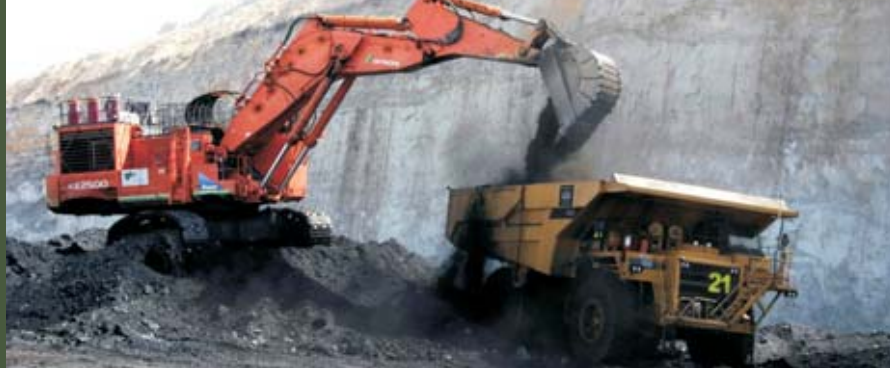
An excavator loading coal.
