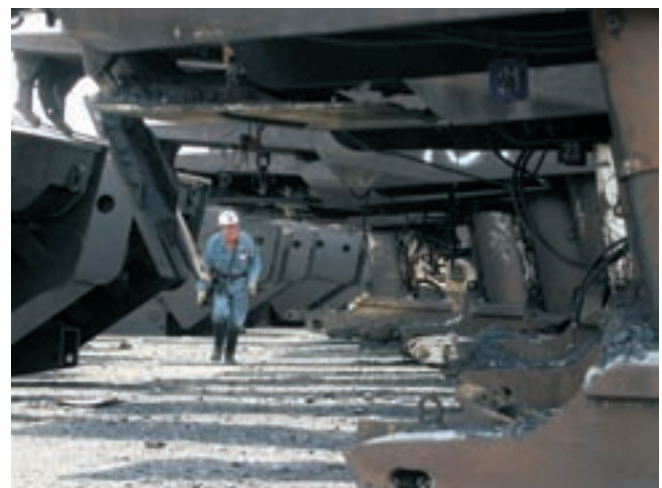
Ian McDonald, Crew Leader, inspecting longwall hydraulic chocks removed from the underground at Dartbrook mine.
