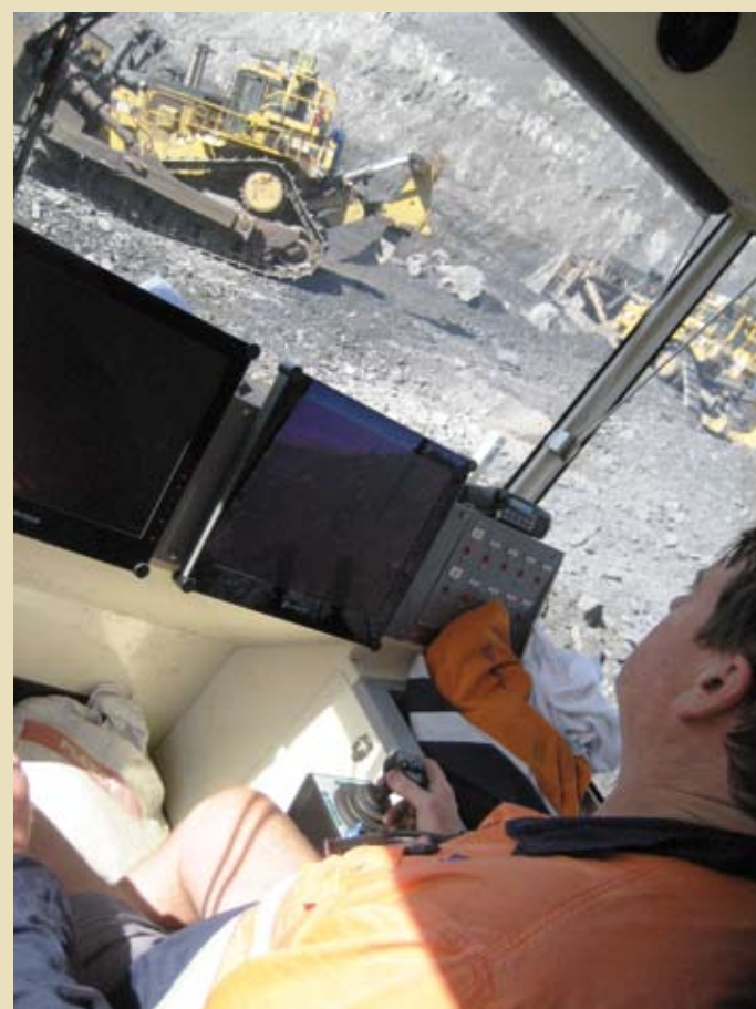
Operator John Tunney handles the control system for the remote ripping of hard rock in the mine pit without exposure to high levels of vibration and jolting
