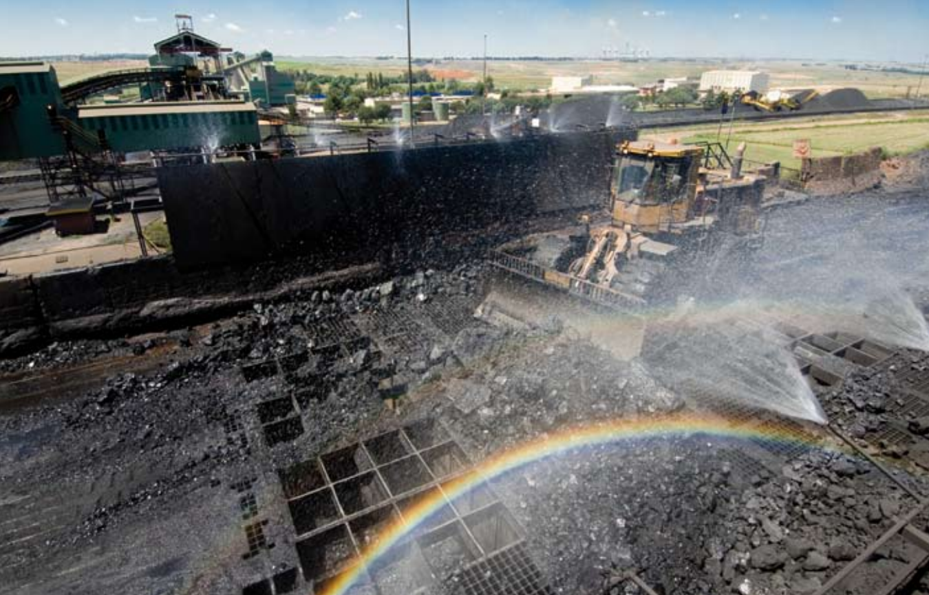
Water jet systems are used to prevent the spread of coal dust from the crushers at the mines
