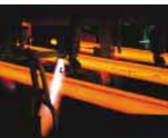
Natural gas-cutting of billets.
