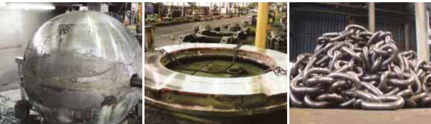
Left and centre: Ball and ring assembly. Right: 36mm long link chain for Portnet.
