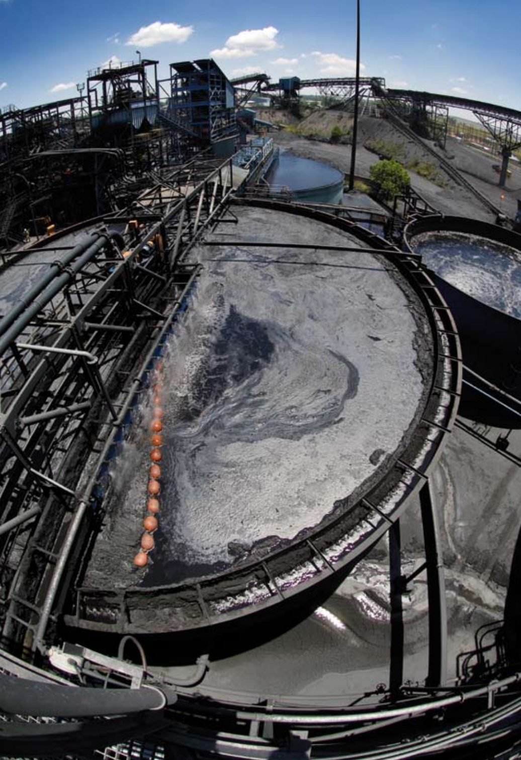
The flotation plant at Greenside colliery recovers valuable ultra-fine product coal.
