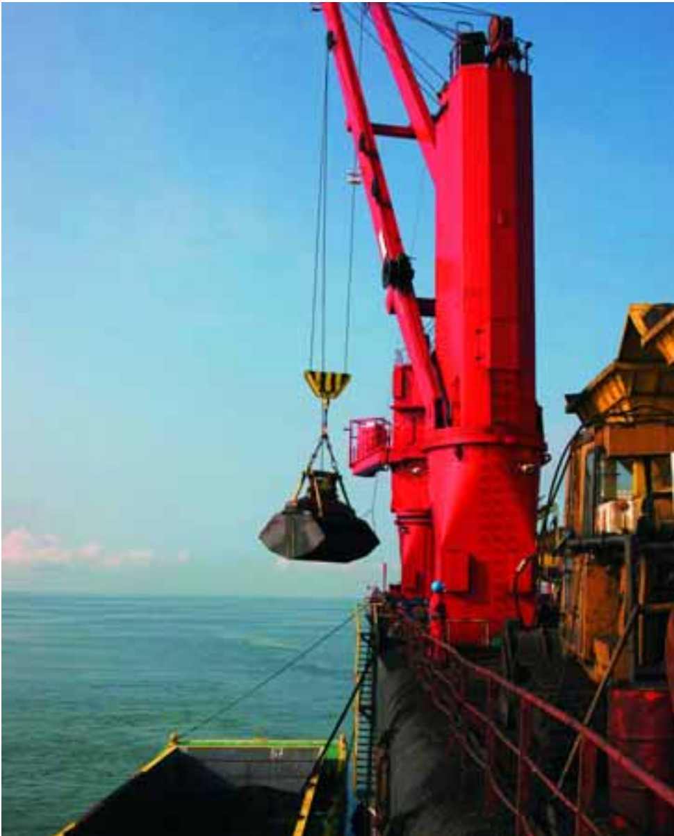
Right: The floating loading facility on Lake Maracaibo. Barges from the port of Santa Cruz bring the coal to the loading facility. Coal from the Paso Diablo mine in Venezuela is loaded here.
