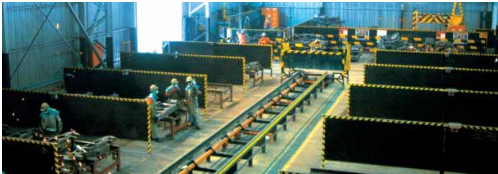
Locomotive frames being machined on one of two new fettling lines at the Germiston machine shop.
