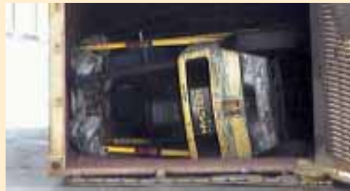
Using a mechanical means as additional support to a trailer.
