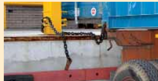
Securing a trailer with a chain.
