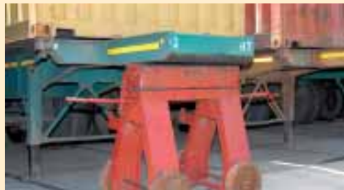
Using a mechanical means as additional support to a trailer.
