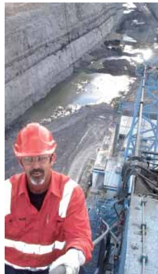
Only trained professional employees may inspect Scaw ropes on dragline booms that rise many metres into the air. Here Haggie Reid Australia technician, Robert Whately, conducts a rope inspection at the boom point on a dragline operating on an open cast mine in Queensland.
