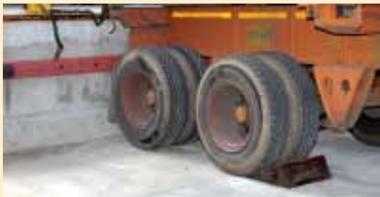
"Chocking" a trailer's wheels to eliminate movement.
