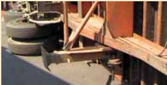
"Chocking" a trailer's wheels to eliminate movement.
