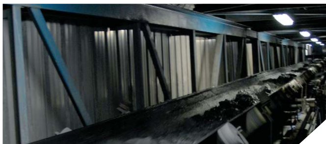
Rock containing lead and zinc from the underground crusher travelling from beneath the enclosed stockpile to the process plant.
