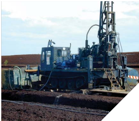
Surface drill rig for drilling exploration holes.
