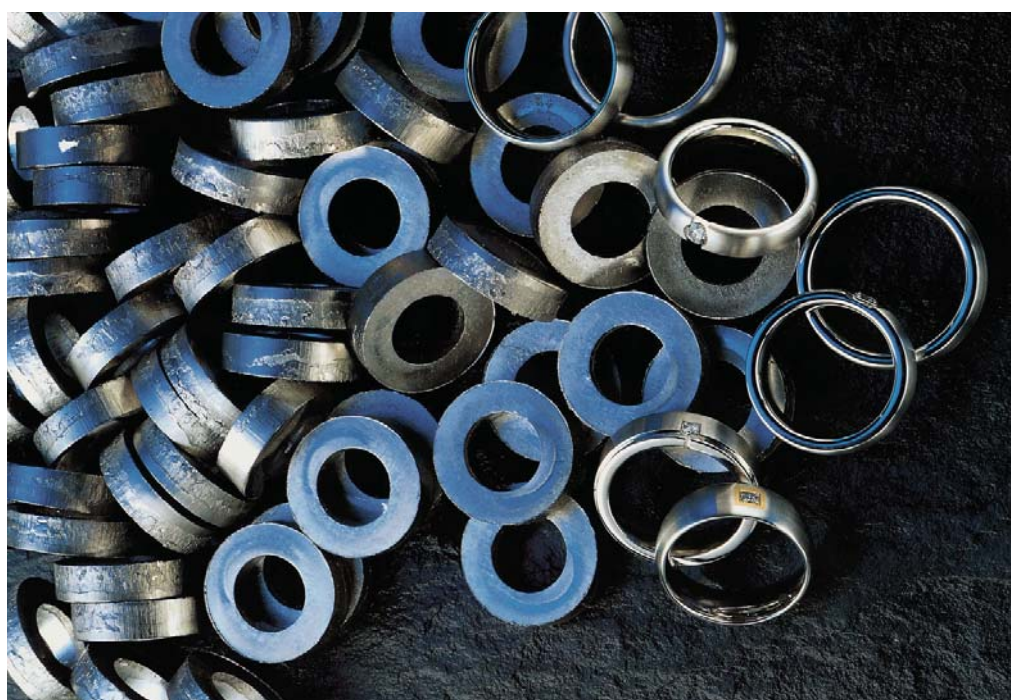
Right: Washers struck from platinum sheet are crafted into bridal rings. Although jewellery remains the No. 2 demand sector for platinum, behind the autocatalyst sector, the metal's use in industry continues to increase and industrial applications now represent nearly a quarter of total demand.
