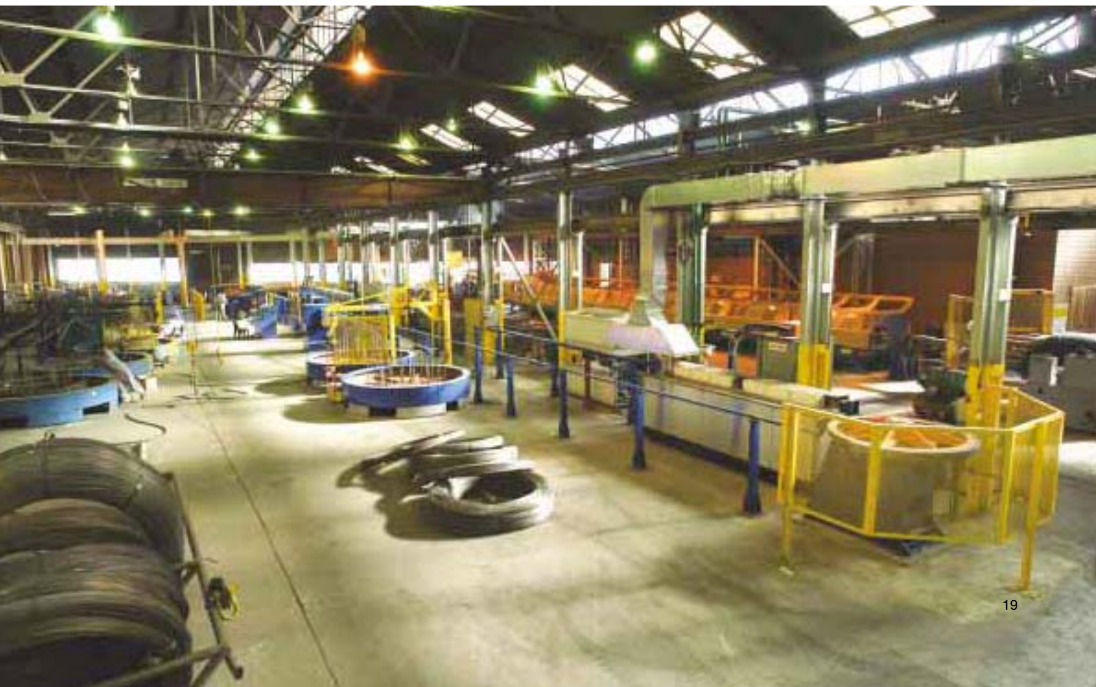
The second low relaxation pre-stressed wire line at the Wire and Strand factory.
