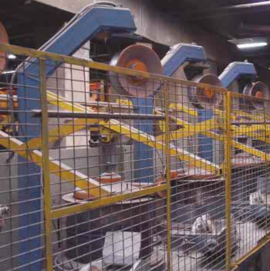
New safety measures have been put in place on wire drawing equipment.
