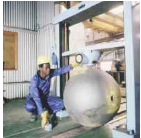
Hardness testing of coal pulverising ball.
