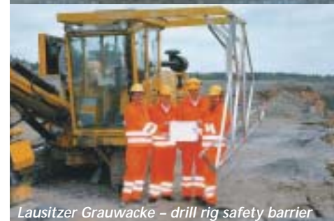
Lausitzer Grauwacke – drill rig safety barrier
