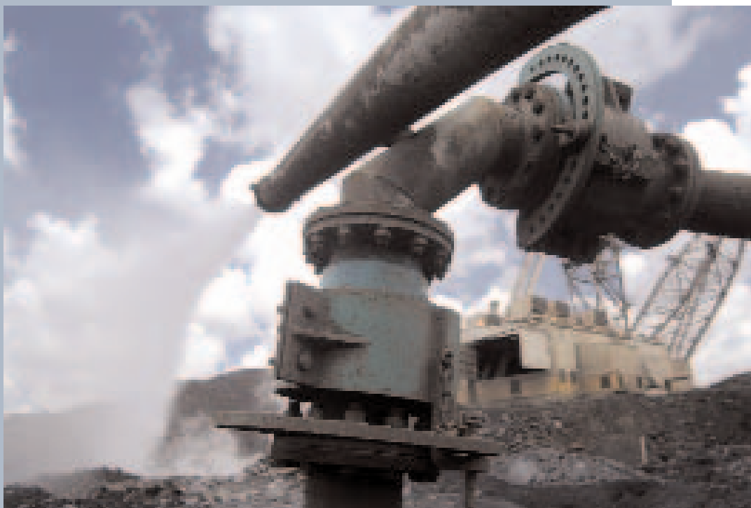
Spontaneous combustion at Kleinkopje is managed using water jets to cool the mined area
