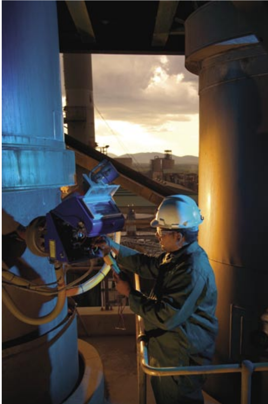
Donovan Rieger monitoring dust at the Waterval Smelter flash dryer unit using the Oaldham laser dust analyzer.
