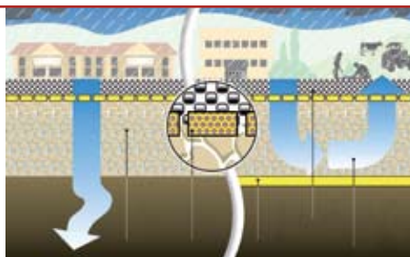
◀ The Aquifa reservoir paving system will help control urban flash floods, by capturing and recycling water.
