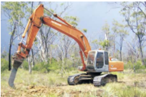
A 24-tonne excavator with the attachment that was developed specifically for Moranbah North Mine subsidence rehabilitation.
