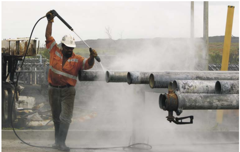
George Tonga, an employee with G & S Engineering, refurbishing water pipes at Moranbah North. This work is carried out on a purpose-built facility which allows the task to be performed safely and the waste material to be contained.
