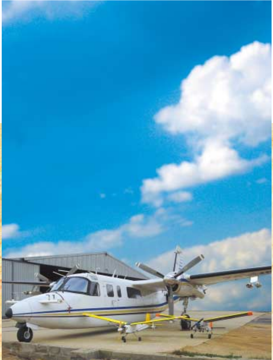
The SA Weather Bureau aero-commander aircraft is equipped with instrumentation for taking multiple air samples, whilst the model planes are used to measure temperature, pressure, humidity and for single air sample trips.
