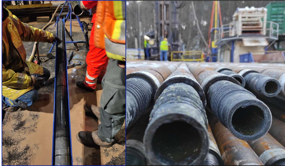
Impressions from the current drilling campaign. On the left the copper shale directly out of the borehole, on the right steel pipes with drill rig in the background.
