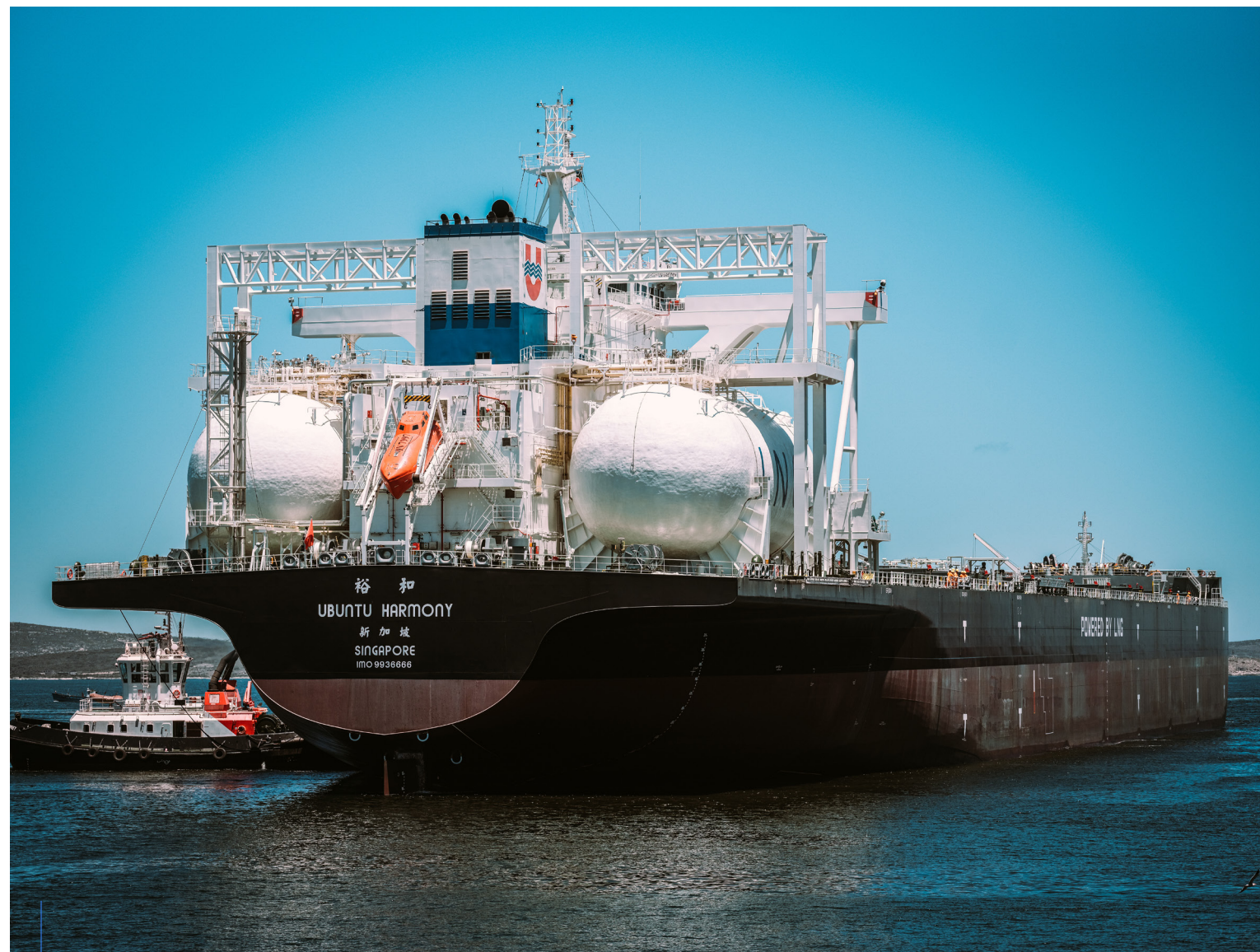
The newly launched LNG dual-fuelled Capesize+ vessel, the Ubuntu Harmony, the inaugural ship in a planned fleet of 10 vessels, with its first cargo of iron ore from Kumba in South Africa. The ships offer significant environmental benefits, with the potential to reach an overall CO 2 emissions reduction of an estimated 35% in comparison with vessels fuelled by conventional marine oil.
