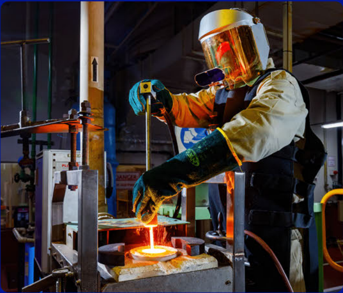
Casting palladium ingots at PGMs’ precious metals smelter at Rustenburg, South Africa.
