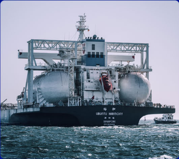
The Ubuntu Harmony is the first of 10 LNG dual-fuelled new-build ships that are already delivering significant reductions in greenhouse gas emissions compared to ships fuelled by conventional marine oil fuel, while also eliminating the release of unburnt methane.
